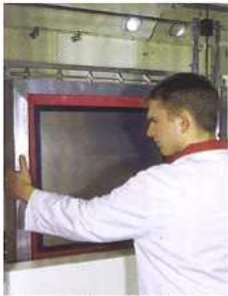
Spider paste and green SMT adhesives are effectively cleaned from framed stencils and foils.
